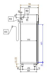
Electrical inlet (power) Refriaerant Inlet Refrigerant Outlet
